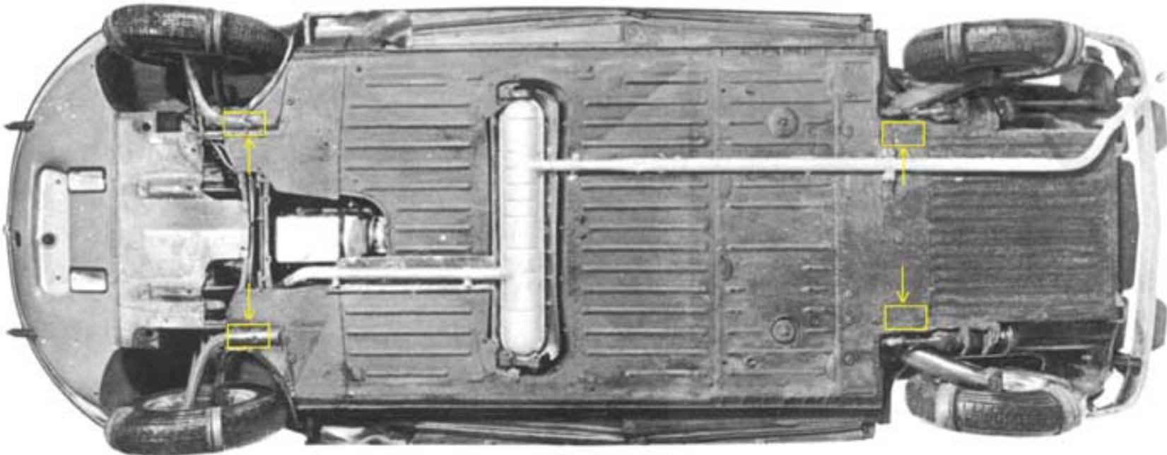
You can use ramps or put the car at the highest position and places stands under the indicated areas. Place a wooden block between the stand and the car to avoid damage in case the car happens to lower itself.
